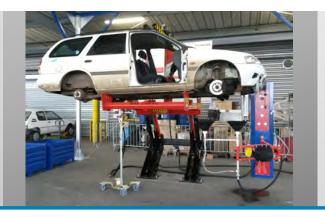
The SEDA TiltingLift TL-2 is a further development of the SEDA TiltingRamp lineup with a unique lifting and tilting feature, which bolts straight to the floor.
