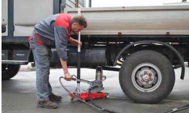
Easy attaching at the tank and drilling
