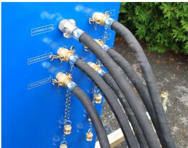
Preinstalled quick couplings for tank line
