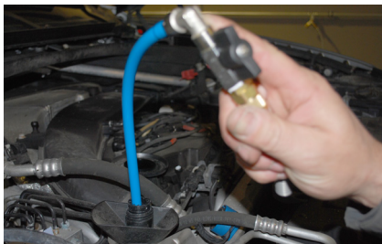
Removal via suction lance into the recovery tank
