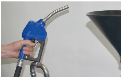
Emptying by nozzle into storage tank.
