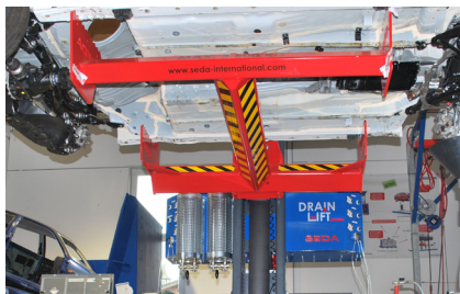
Easy access to vehicles underside due to H-design
