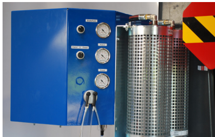
Pump housing with quality control for petrol and diesel
