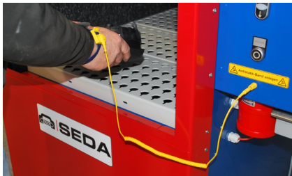
ESD wrist strap for potential equalization
