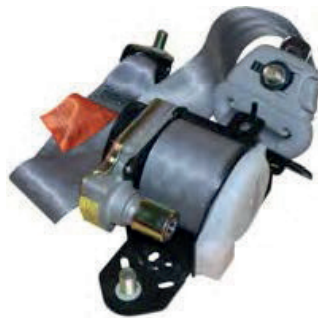
Neutralized belt tensioners
